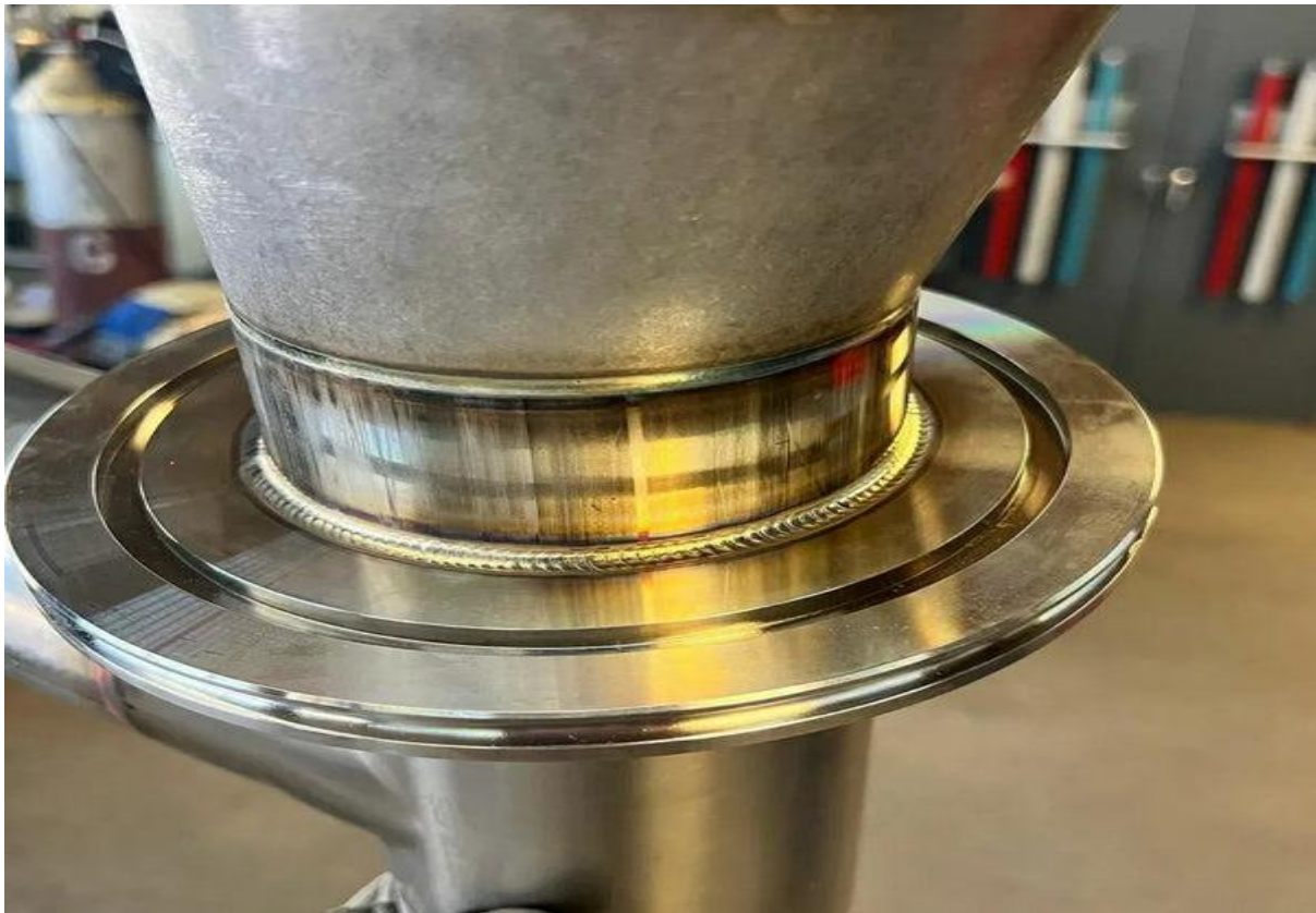
Figure 1. GTAW setup employed for fabrication of stainless-steel weld joints.
